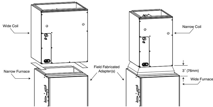
\* CAUTION: DO NOT MOUNT COIL LOWER THAN 3" (76mm) MINIMUM OR FURNACE FAILURE MAY RESULT
